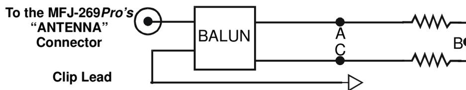
A properly designed **current balun** is the type most effective for maintaining current balance. It has the highest power capability and lowest loss for given materials. It should show a low SWR over the entire operating range of the balun with the clip lead in *any* of the three positions.
